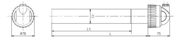
The heaters are designed to be mounted vertically in the tank and will occupy the minimum amount of space. The heater should be mounted on the flange of the tank using the optional hanging bracket. It should be position so the hot zone of the element (marked on the casing) is always below the liquid. It is available in sizes 1kW to 4.5kW in single or three phase with a head to IP65 and flying lead for easy connection leaving no exposed joints near surface.
