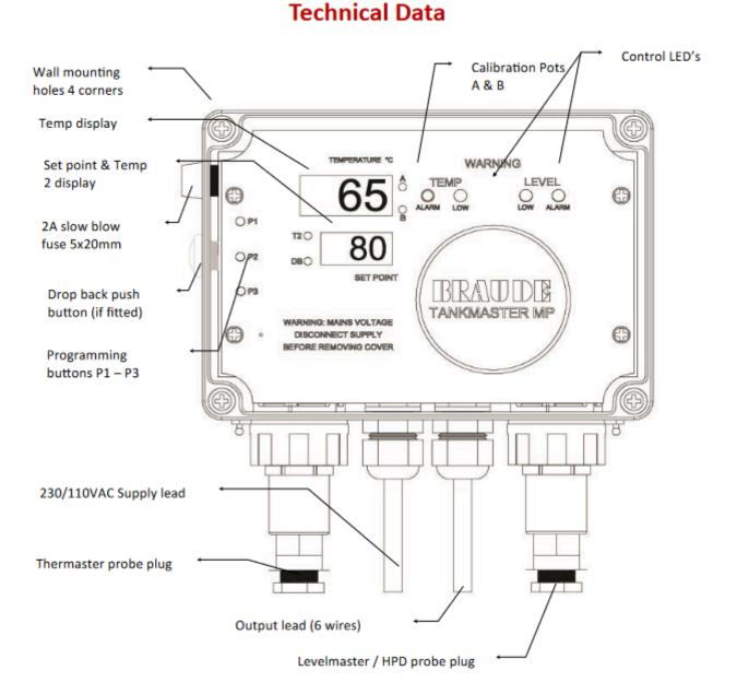
Enclosure to IP65, surface mounted, supplied with 1 metre flying leads. Dimensions 175mm x 125mm x 75mm deep.
