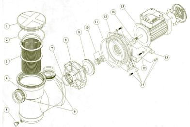
The Braude Self Priming Pump is reliable, and easy to maintain. We hold a large stock of spare parts and all pumps are supplied with clear installation, operating and maintenance instructions, and Braude technical staff are always available to offer advice.
