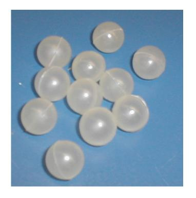
Frogspawn consist of hollow spheres which are floated on the top of the tanks covering up to 90% of the surface reducing heat loss and vapour losses thereby improving the working environment. Availability in a variety of sizes and resistant to virtually all the solutions used in the industry eg acid, alkalis inorganic and some organic.
