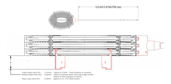
All units min 50mm of solution above heater height. Hangers and standoffs are supplied with the heater. Add 12.5mm and 25mm respectively to above thicknesses. Baffles are supplied as optional extra.
